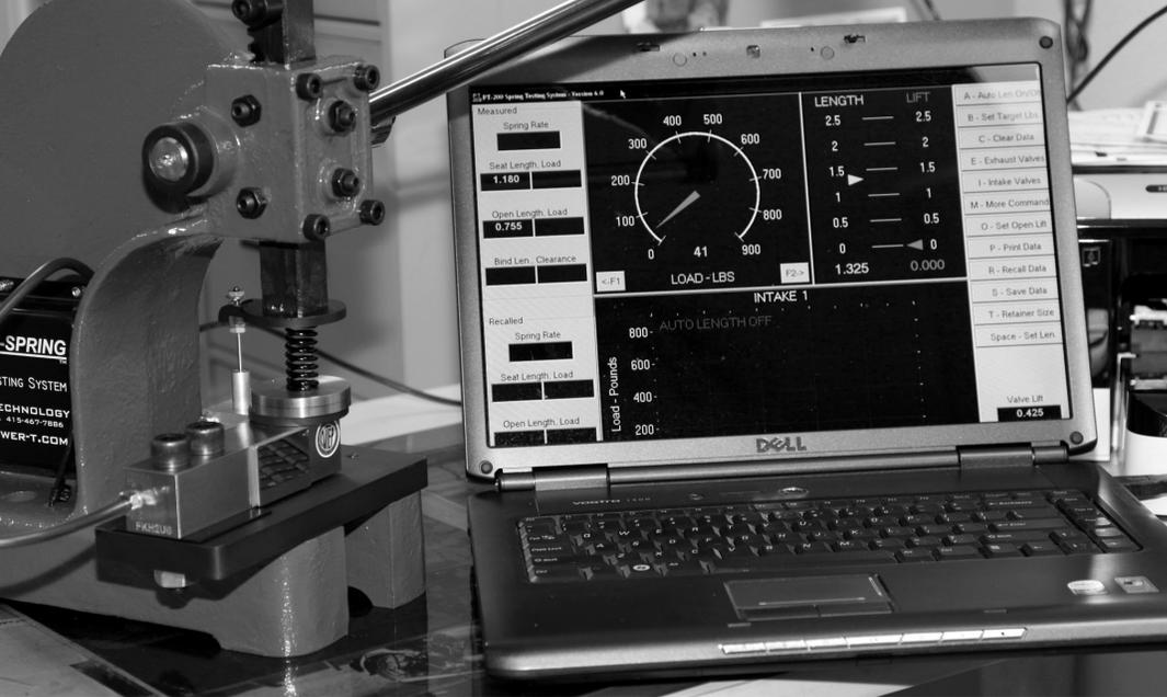
Sampling various clutch springs using a PT-200 Valve Spring Tester. This is a 57-1830 spring and you can see on the PC screen 42 lb. at 1.325".
